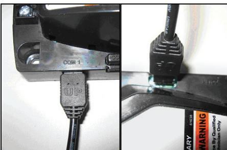
Contractor Tool cord must be oriented as shown for proper operation.
