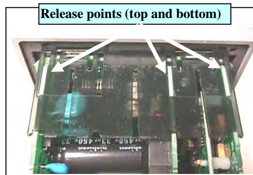
Figure 3 Removing Printed Circuit Boards
