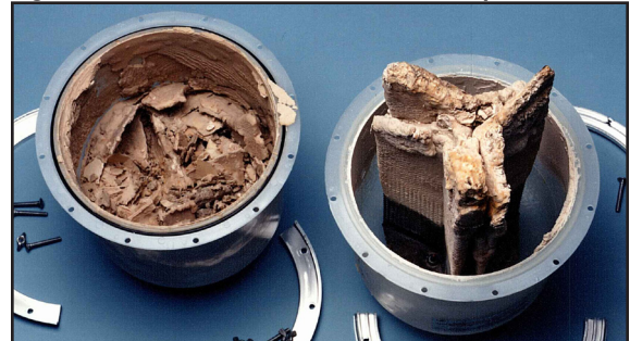
Figure 23-1. Tank filled with mineral buildup.
