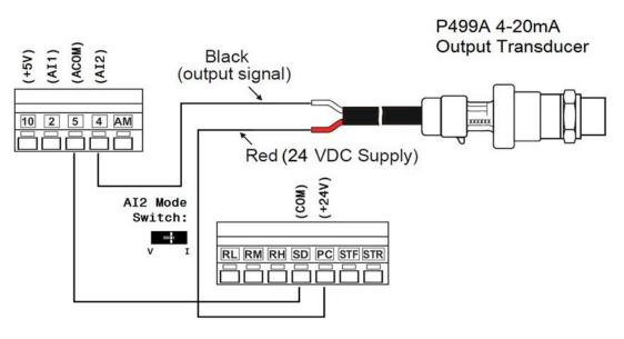
Figure 17: Wiring a 4–20 mA Input Signal Transducer
