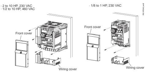
Figure 6: Mounting the VFD68 Drive
