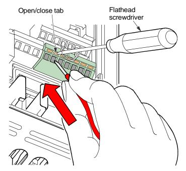
Figure 14: Wiring Analog Input Devices to the VFD68 Control
