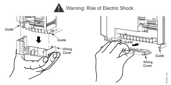
Figure 10: Remove the High-Voltage Wiring Cover
