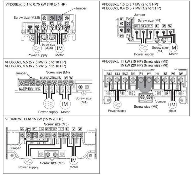
Figure 11: High-Voltage Terminal Block Wiring
