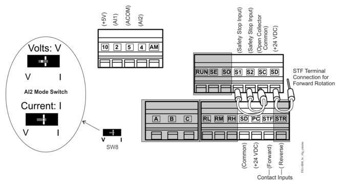
Figure 12: VFD68Bxx and VFD68Cxx Drives Low-Voltage Connections
