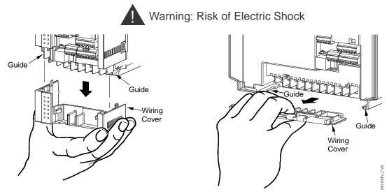
Figure 5: Remove the High-Voltage Wiring Cover
