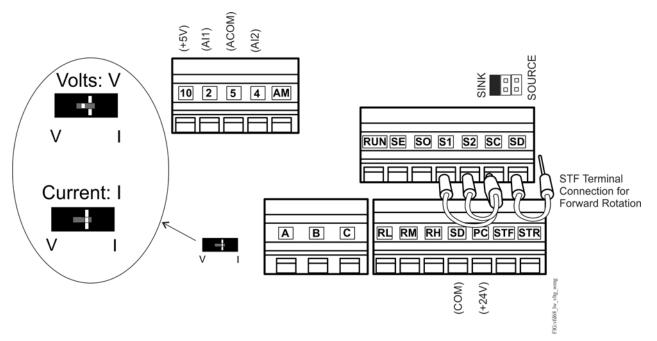
Figure 24: VFD68 Setup and Low-Voltage Connections
