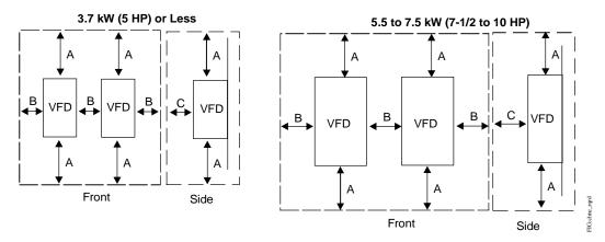
Figure 7: Required Clearance for Mounting Inside an Enclosure
