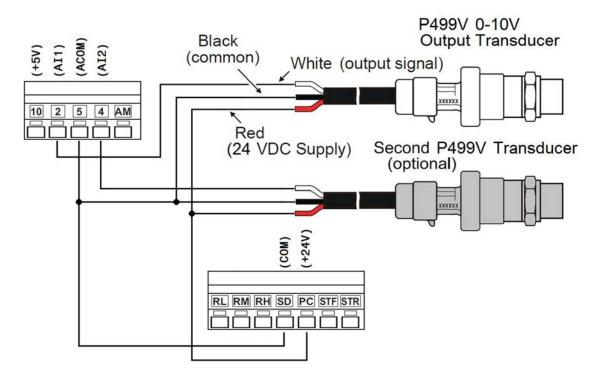
Figure 16: Wiring 0–10 VDC Input Signal Transducers
