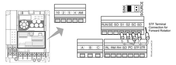
Figure 13: Locating the Low-Voltage Wiring Terminals
