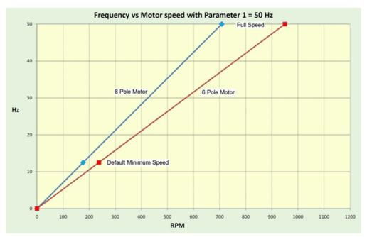
Figure 20: Frequency and Motor Speed (50 Hz)
