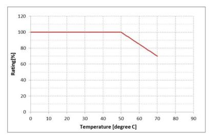
Figure 2: VFD68Bxx and VFD68Cxx Maximum Current Output Derating above 50°C
