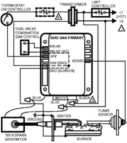
A POWER SUPPLY, PROVIDE DISCONNECT MEANS AND OVERLOAD PROTECTION AS REQUIRED.
