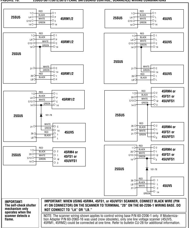
**Note 1:** Diode part No. 101-78 must be connected as shown in signal lead (14) of the 45UV5 scanner when using with a 45RM, 45FS, or 45UVFS scanner.
