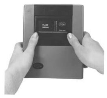
To remove the cover, place your fingers and palms on each side and pull forward as shown in the diagrams. Press down with thumbs while pulling out with your palms and fingers. The cover will snap off and can be snapped back into place easily.
