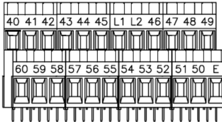
**The fuel select switch connects to terminals 45, 49 and 53.**
